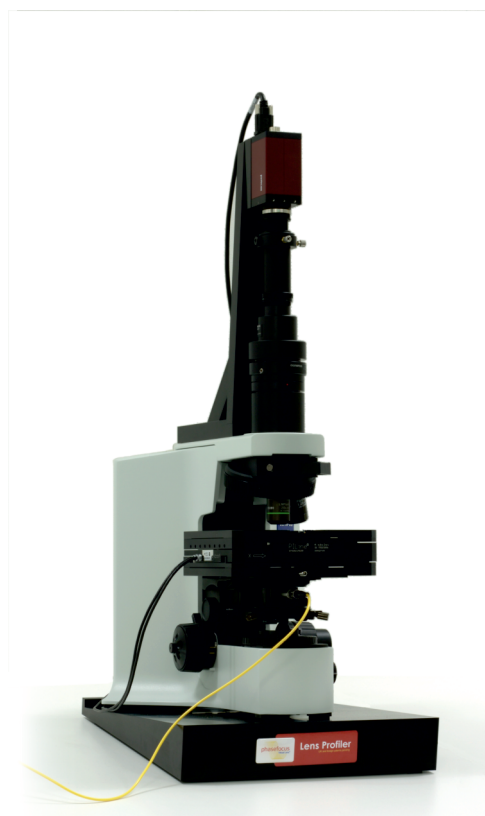
Figure 1: Contact lens measurement system based on a standard optical microscope.
